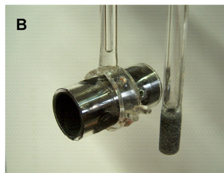
Fig. 3. (A) Simplified reaction pathways of the hydrogenation of cinnamaldehyde. The products reactions are the hydrocinnamaldehyde, the cinnamyl alcohol and the 3-phenyl-1-propanol. (B) Optical image showing the fixation of the catalyst which was subsequently used as stirrer.
